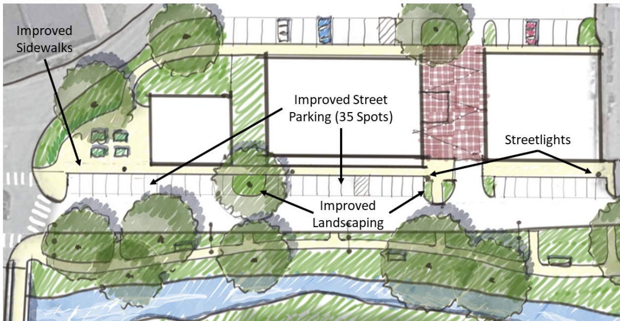
Main Street Improvements Including an Improved Parking Lot, Streetlights, Landscaping, and Sidewalks
