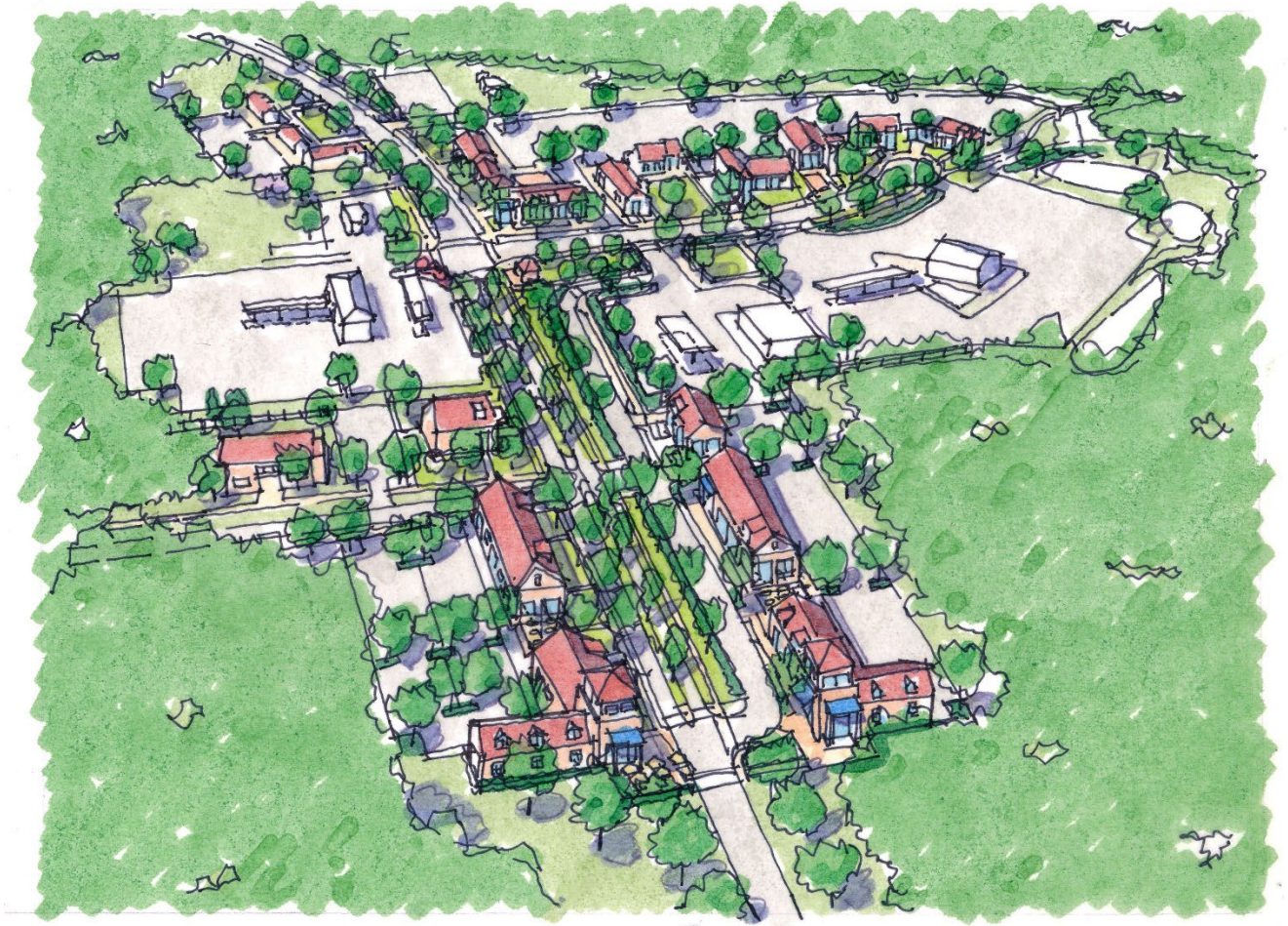
“Gas Backwards”: example interchange commercial area showing buildings placed towards road to screen gas pumps in the rear, and parkway plantings.
