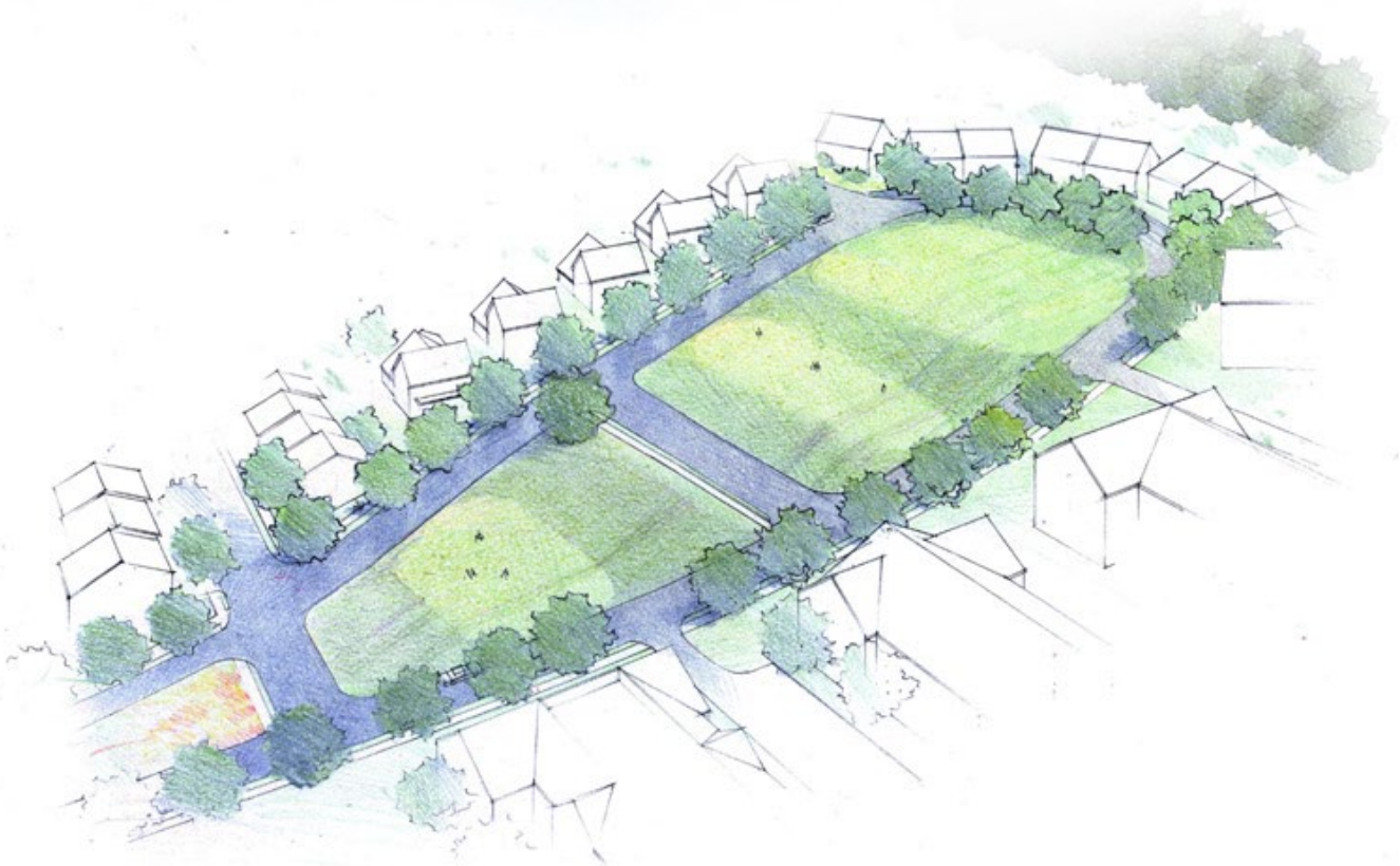
Example: lot sizes reduced to 15,000 SF around edges of a common that doubles as stormwater management facility
