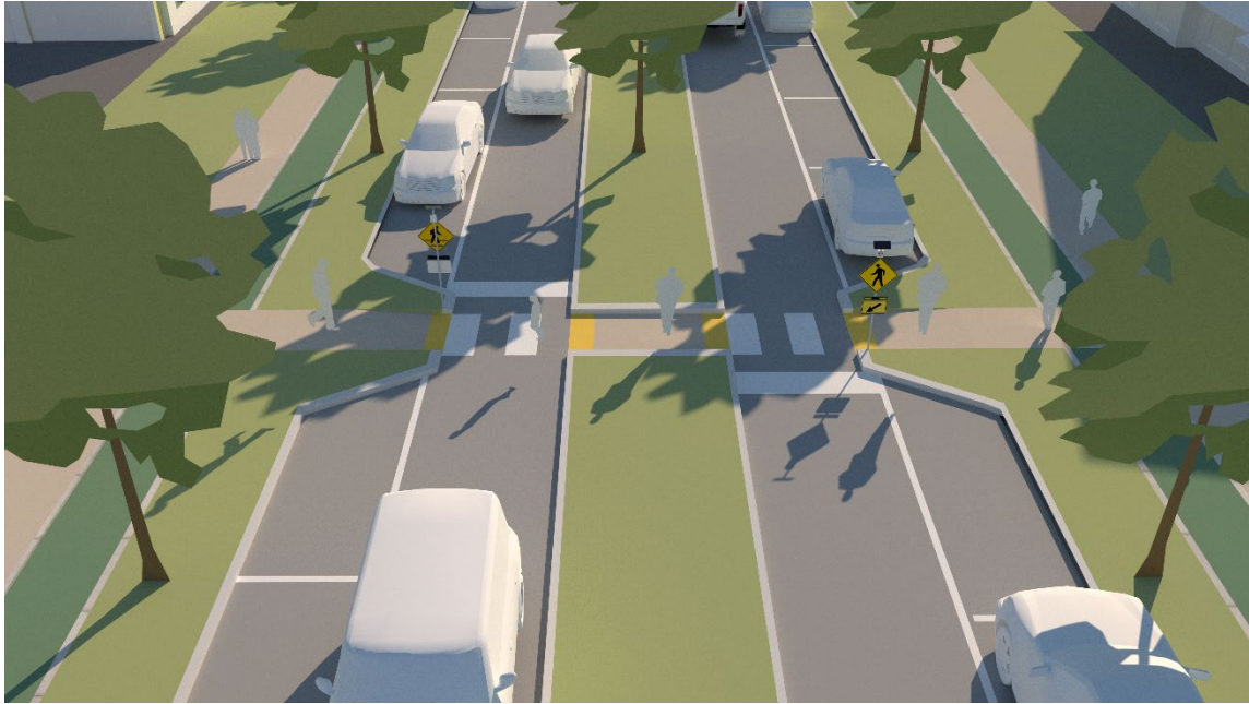
Minor Street Crossing – 3/4 View
